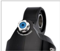
Nitrogen gas valve
